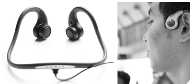
Figure 1. Bone vibrator(Huria Inc., HUH-701) used for tinnitus retraining therapy(TRT).
